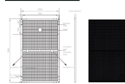
Module dimensions in the technical picture are expressed in mm with tolerance ±2 mm (±0.079 °) 1 - Standard Test Conditions (STC): Irradiance 1000 W/m<sup>3</sup>, Air Mass AM = 1.5, Cell Temperature 25°C); Tol
